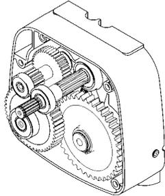
**Figure 6 - Assembled Gearing**
