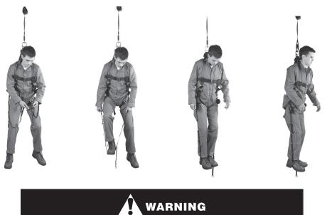
The RL-TRP is a temporary stress relief system. Rescue must be prompt. Do not adjust any harness buckles while using the RL-TRP.
