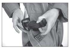
4. Insert the RL-TRP pack through its own web loop and pull snug to create a web choke attachment.
