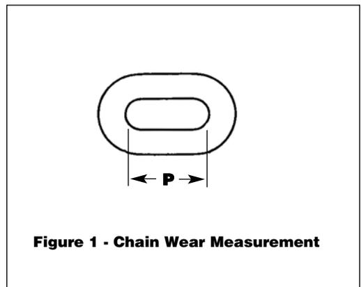
**Figure 1 - Chain Wear Measurement**
