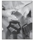
Adjust all keepers, buckles, padding, and D-ring to inspect webbing hidden by these components.
