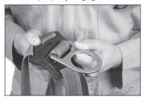
Tongue buckle/grommet tongues should be free of distortion in shape and motion. They should overlap the buckle frame and move freely back and forth in their socket. The roller should turn freely on frame. Inspect for loose, distorted, or broken grommets. Webbing should not have additional punched holes.
