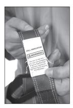
If inspection reveals any defect, inadequate maintenance, or unsafe condition, remove from service immediately. Any harness with noticeable wear or damage must be removed from service immediately. Contact Rigid Lifelines for help with replacement.
