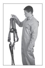
Slip shoulder strap over one shoulder, then pull the other shoulder strap 2. around the back and over the second shoulder — much like putting on a jacket. The dorsal D-ring will be located on your back while the chest strap is located in the front. Straps must not be tangled as the harness hangs freely from shoulders.
