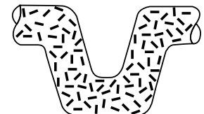
CASTING Random grain flow with larger grain structure makes material weaker than forged products
