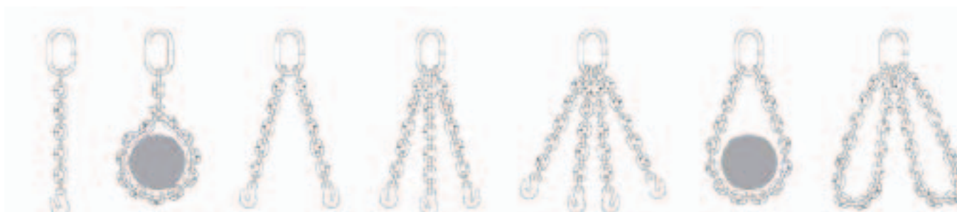
SINGLE LEG (VERTICAL) SINGLE LEG (CHOKER) DOUBLE (2 LEGS) TRIPLE (3 LEGS) QUADRUPLE (4 LEGS) BASKET TYPE DOUBLE BASKET TYPE
