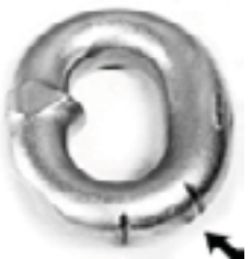
Figure 2: Location of nicks, gouges, and notches will dictate their severity.
