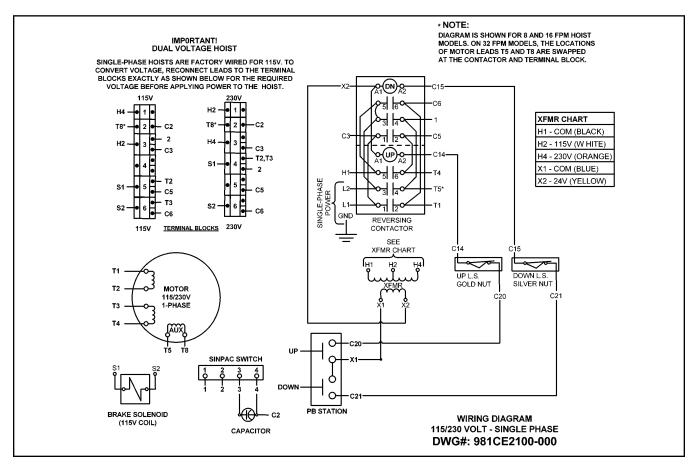
Figure 9A — Wiring Diagram for 115/230V - 1 Phase Models
