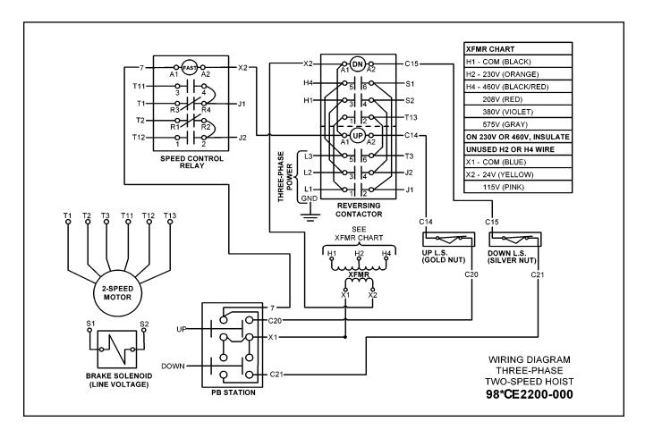
Figure 9D — Wiring Diagram for 2-Speed, 3 Phase Models \* Factory supplied diagrams will be numbered beginning with 98<u>3</u> for 230 or 460V, 98<u>5</u> for 575V, 98<u>7</u> for 208V, and 98<u>8</u> for 380V.
