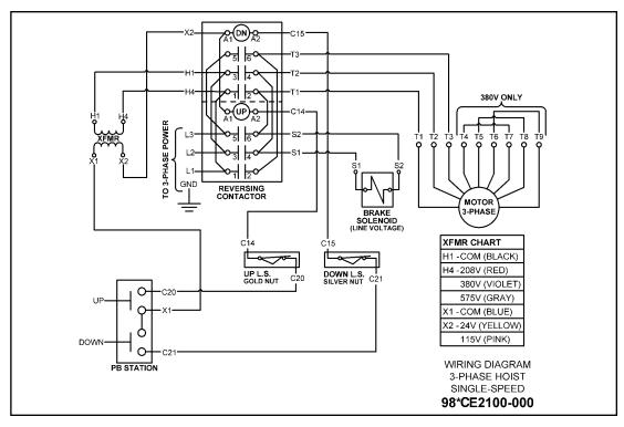
Figure 9C — Wiring Diagram for 1-Speed, 208V, 380V, 575V - 3 Phase Models \* Factory supplied diagrams will be numbered beginning with 985 for 575V, 987 for 208V, and 988 for 380V.
