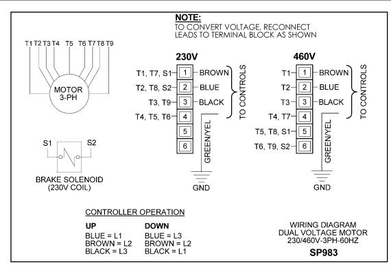
Figure 9A — Wiring Diagram
