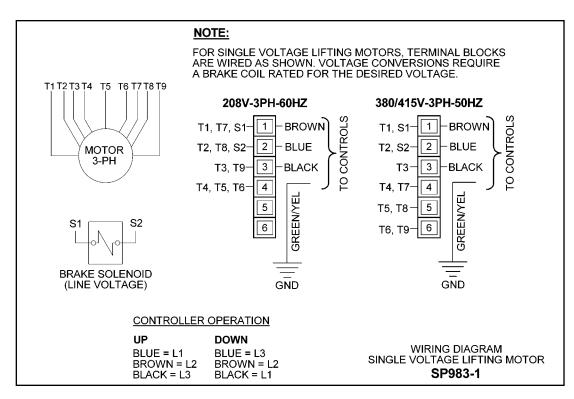
Figure 9B — Wiring Diagram
