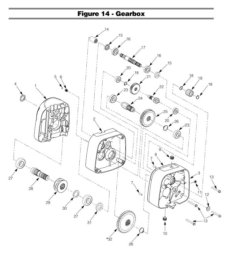
\*NOTE: Orient output gear (32) with long boss towards gearbox cover (3).
