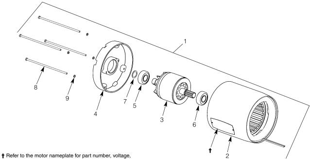
Refer to the motor nameplate for part number, voltage, full load amperage, horsepower, and other motor information.
