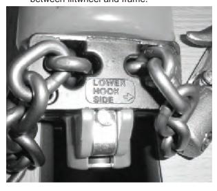
Figure 12. Chain Assembly - Hook End, 3/4 Ton
