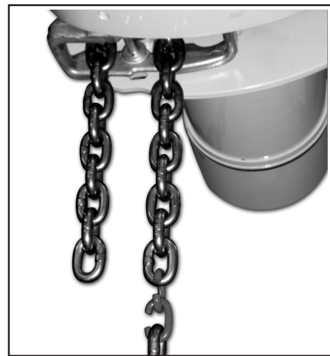
Figure 5-4. Installing Coil Load Chain Using Two "C" Links (1/4, 1/2 & 1 ton hoists)
