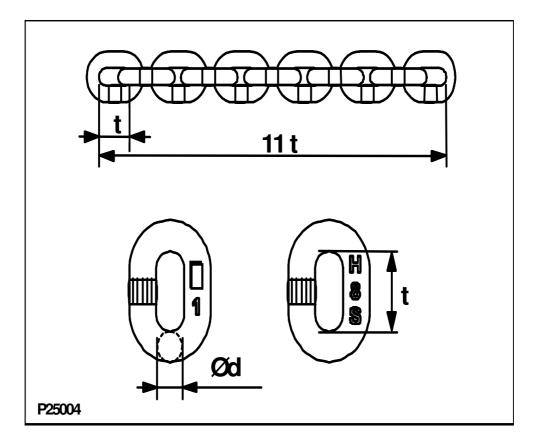
Measure the following chain dimensions at several points on chain: (Figure 12)
