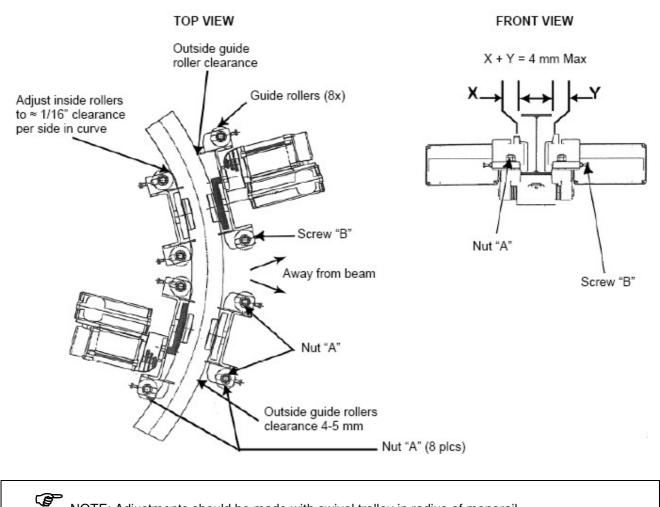
NOTE: Adjustments should be made with swivel trolley in radius of monorail.
