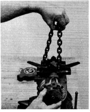
INSTALLING LOAD CHAIN FIGURE 5
