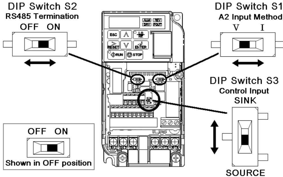
*Figure 3-5: DIP Switches*
