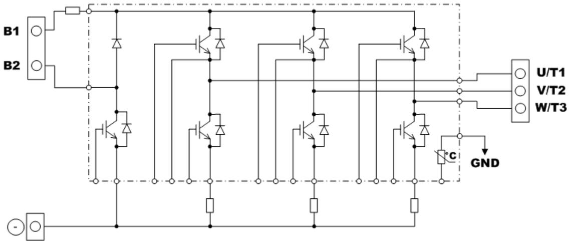
*Figure 6-1: Braking Circuit*
