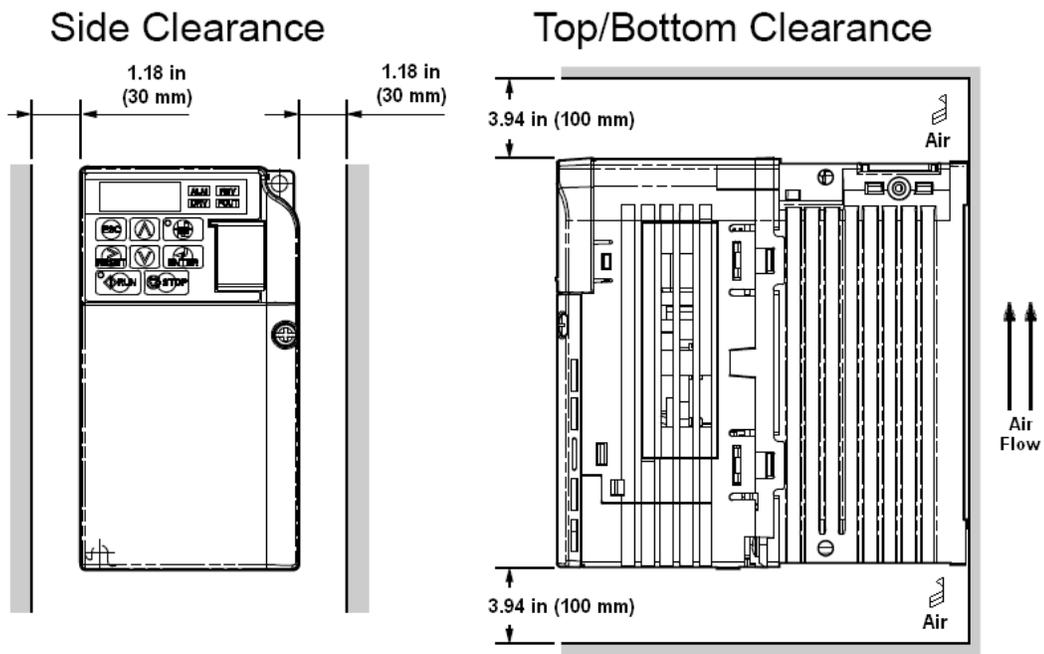
*Figure 2-2: Standard Installation*
