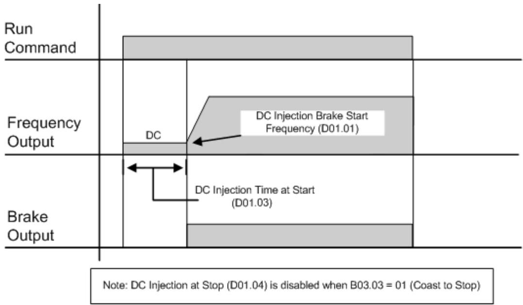
Figure 5-3: B03.03 = 00 (Decel to Stop) with DC Injection
