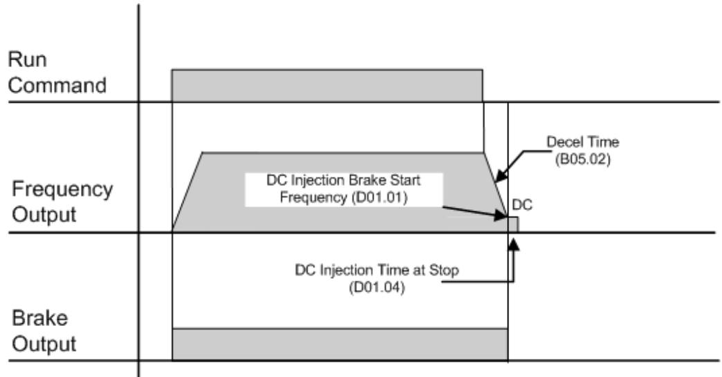
Figure 5-2: B03.03 = 00 (Decel to Stop) without DC Injection
