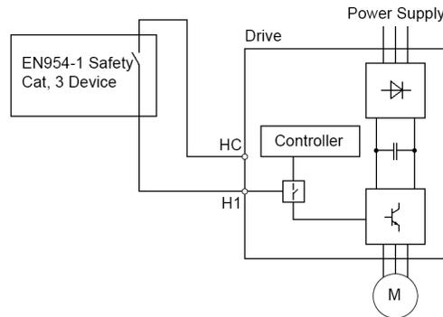
*Figure 3-2: Safe Disable Wiring Example*
