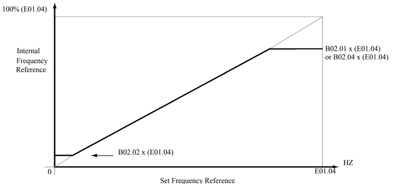
**Figure 5-1: Setting Frequency Upper and Lower Limits**
