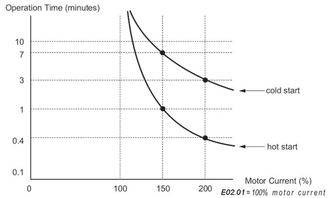
**Figure 5-13: Motor Protection Operation Time**
