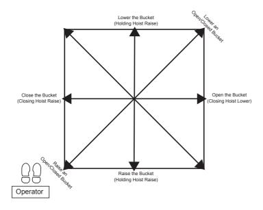
This new custom software can be used with IMPULSE•VG+ Series 3 drives to control multi-line clamshell or grapple buckets that utilize a loading/closing hoist. Although the open and hold drive operate independently, the software lets you control the various motions of the bucket without the need for a PLC.
