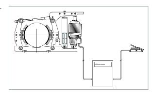
Improved torque control ensures a smooth transition from coasting to slowing down and is non-destructive to the controls or the crane itself. As more torque is applied, the crane will accelerate or decelerate faster. An optional input to the drive while the footbrake is applied prevents the motor from driving into the brake, saving wear and tear.
