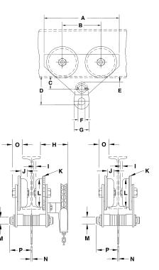
Note: Wheels with convex treads are standard on all capacities 1/4 - 20. 20, 25, 30 and 40 ton trolleys can be furnished in tandem construction - Dimensions for 30 thru 50 ton upon request. Dimensions shown are for minimum beam size and will vary proportionately for larger beams.
