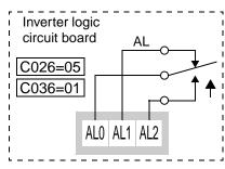
Relay shown with inverter power ON, Alarm Signal OFF
