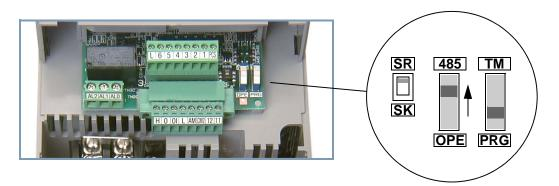
At this point the electrical network connection is complete. The next step will show how to configure parameters and settings related to ModBus communications.
