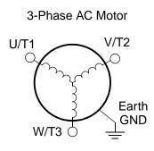
cause equipment damage or personnel injury, be sure to verify direction of rotation before attempting full-speed operation. For safety to personnel, you must connect the motor chassis ground to the ground connection at the bottom of the inverter housing.
