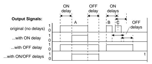
To configure ON and OFF delays, use the following table to set the desired delay times.
