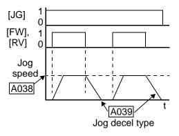
The type of deceleration used to end a motor jog operation is selectable by programming function A039. The options are:
