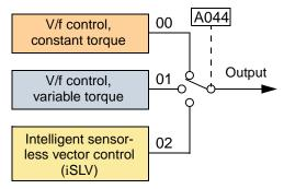
mode. Use A044 to select the torque control algorithm as shown in the diagram. The Sj200 inverter's iSLV mode eliminates the need for manual entry of additional motor parameters, or even for doing an auto-tuning procedure.
