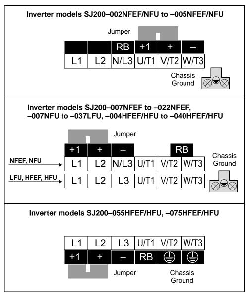
**NOTE:** An inverter powered by a portable power generator may receive a distorted power waveform, overheating the generator. In general, the generator capacity should be five times that of the inverter (kVA).
