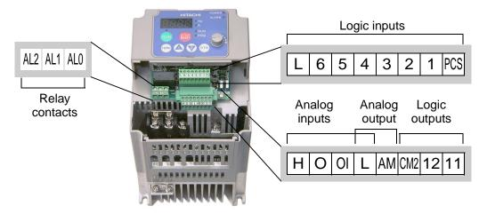
Specifications for the logic connection terminals are in the following table:
