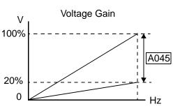
**Intelligent Sensorless Vector Control (iSLV)** – This advanced torque control algorithm improves torque performance at very low speeds—down to 0.5 Hz, as well as improve regulation across the speed range. Set parameter A044=02 to select iSLV operation. The iSLV algorithm automatically matches the characteristics of the particular motor connected to your inverter. Auto-tuning is not required. The iSLV control includes voltage compensation (A046) and slip compensation (A047).
