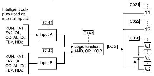
The following table shows all four possible logic input combinations with each of the three available logical operations.
