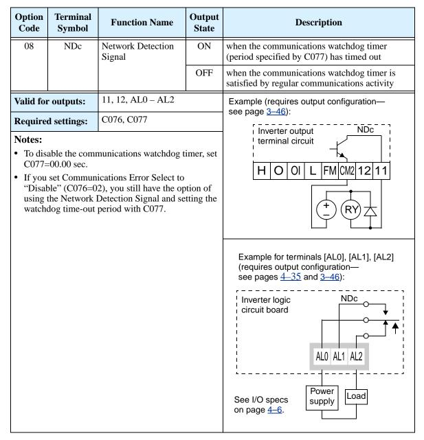
Additionally, the inverter can respond to a communications time-out in various ways. Refer to the following diagram (top of next page). You configure the desired response via function C076, Communications Error Select. This selects whether or not you want the inverter to trip (alarm with error code E60) and whether to stop the motor or just let it coast. Together, parameters C076 and C077 set the network detection watchdog time-out and the inverter's response.
