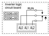
Relay shown with inverter power ON, Run Signal OFF
