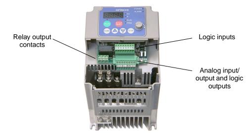
**Logic Connector Removal/Replacement -** The two 8-position main logic connectors are removable from the circuit board to make testing or service more convenient. Note that the relay output connector is not removable, as it must carry higher currents and provide high integrity for alarm conditions. The alarm circuit may carry hazardous live voltages (from external wiring) even when the main power to the inverter is OFF. So, never directly touch any terminal or circuit component.
