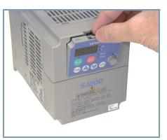
**Internal LED Indicators / Communications Connector -** Refer to the keypad bay in the illustration below. After removing the keypad, the internal LED viewing window will be visible. These LEDs indicate status for your convenience when the keypad is remotely mounted and you are nearer to the inverter location.
