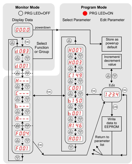
The navigational map shows the relationship of all resources of the inverter in one view. In general, use the  $\bigcirc$  key to move left and right, and the  $\land$   $\checkmark$  (arrow) keys to move up and down.
