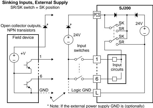
connected to [L], then install the above diode.
