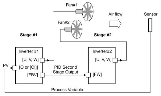
To use the PID Second Stage Output feature, you will need to choose upper and lower limits for the PV, via C053 and C052 respectively. As the timing diagram below shows, these are the thresholds Stage #1 inverter uses to turn ON or OFF Stage #2 inverter via the [FBV] output. The vertical axis units are percent (%) for the PID setpoint, and for the upper and lower limits. The output frequency, in Hz, is superimposed onto the same diagram.
