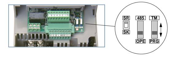
The TM/PRG switch setting forces terminal operation, according to the table below:
