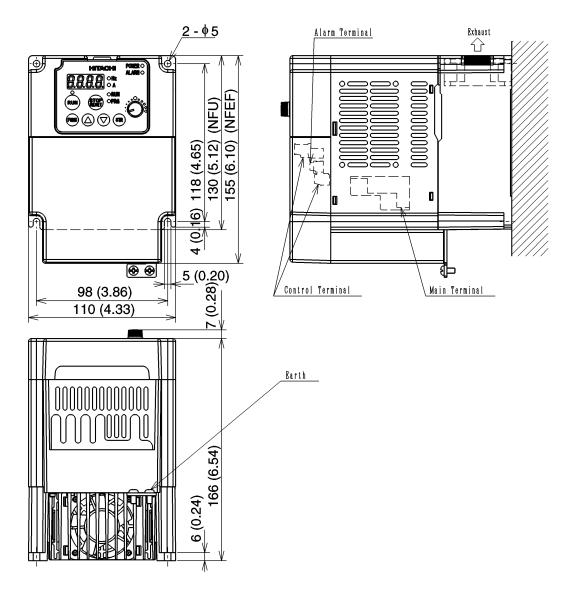
Inverter Mounting and Installation
