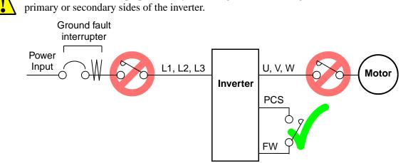
CAUTION: Do not stop operation by switching OFF electromagnetic contactors on the
