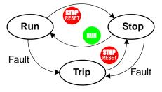
either case, you can clear the fault by pressing the Stop/Reset key. Additionally, you can clear the inverter's cumulative trip history by performing the procedure <u>"Restoring</u> <u>Factory Default Settings" on page 6–8</u> (setting B084=00 will clear the trip history but leave inverter settings intact).
