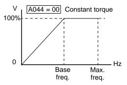
**Manual Torque Boost** – The Constant and Variable Torque algorithms feature an adjustable *torque boost* curve. When the motor load has a lot of inertia or starting friction, you may need to increase the low frequency starting torque characteristics by boosting the voltage above the normal V/f ratio (shown at right). The function attempts to compensate for voltage drop in the motor primary winding in the low speed range. The boost is applied from zero to 1/2 the base frequency. You set the
