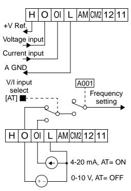
**NOTE:** If no logic input terminal is configured for the [AT] function, then inverter sums the voltage and current input to determine the desired input value.
