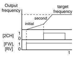
In the graph shown above, the [2CH] becomes active during the initial acceleration. This causes the inverter to switch from using acceleration 1 (F002) to acceleration 2 (A092).
