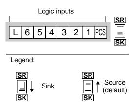
**CAUTION:** Be sure to turn OFF power to the inverter before changing the SR/SK switch position. Otherwise, damage to the inverter circuitry may occur.
