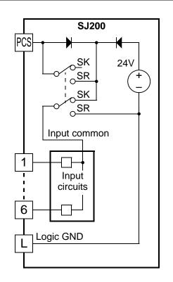
The two diagrams below show input wiring circuits using the inverter's internal +24V supply. Each diagram shows the connection for simple switches, or for a field device with transistor outputs. Note that in the lower diagram, it is necessary to connect terminal [L] only when using the field device with transistors. Be sure to use the correct SR/SK switch position shown for each wiring diagram.
