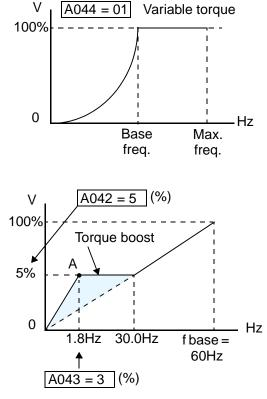
breakpoint of the boost (point A on the graph) by using parameters A042 and A043. The manual boost is calculated as an addition to the standard V/f curve.
