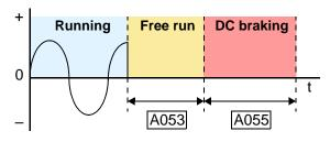
during deceleration below a frequency you can specify (A052). The braking power (A054) and duration (A055) can both be set. You can optionally specify a wait time before DC braking (A053), during which the motor will free run (coast).
