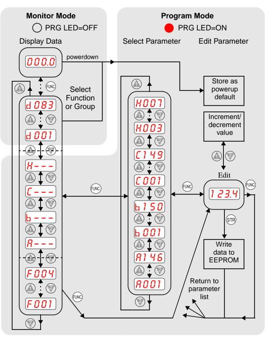
**NOTE:** The inverter 7-segment display shows lower case "b" and "d," meaning the same as the upper case letters "B" and "D" used in this manual (for uniformity "A to F").
