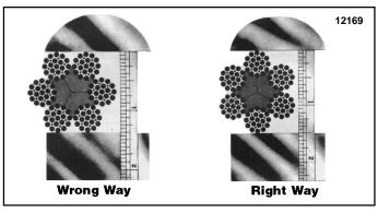
Figure 5-4. Correct Method of Measuring Rope
