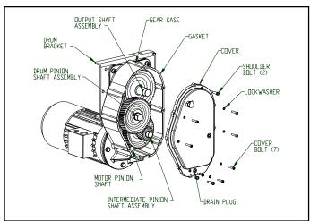
Figure 5-7. Hoist Gear Case Assembly
