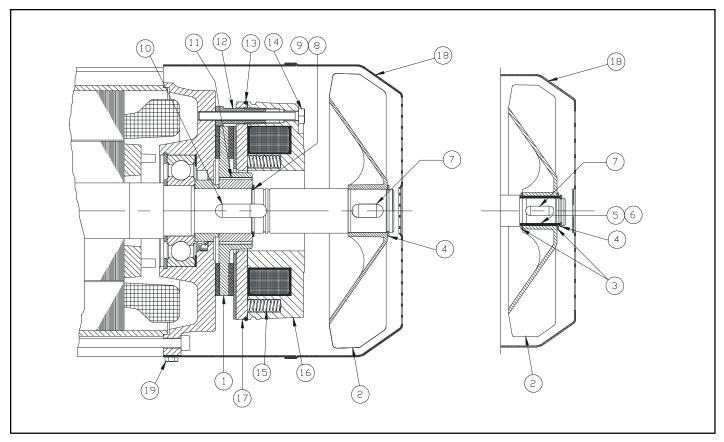
Figure 9-8. Standard Hoist Motor Brake
