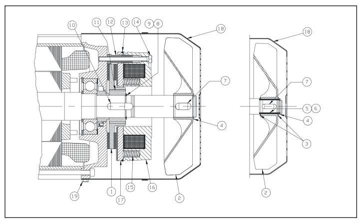
Figure 9-8. Standard Hoist Motor Brake
