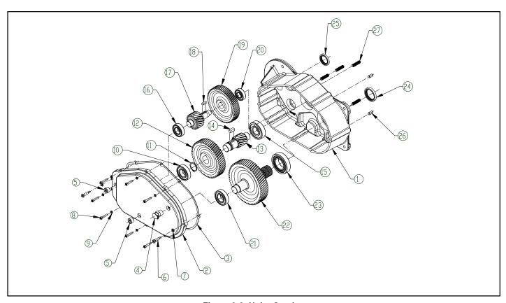
Figure 9-2. Hoist Gearing
