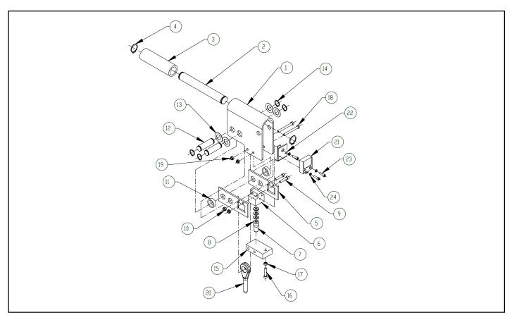
Figure 9-6. Wire Rope Dead End Assembly
