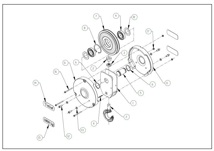
Figure 9-4b. Lower Block Assembly (S2 Reeved)
