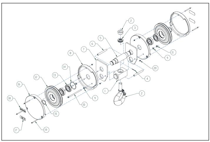
Figure 9-4a. Lower Block Assembly (S4 Reeved)
