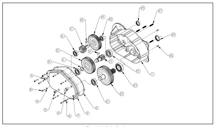
Figure 9-2. Hoist Gearing
