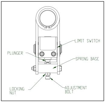
Figure 7-3. Over-Capacity Limit Switch
