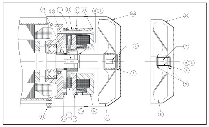
Figure 9-9. Outdoor Service Hoist Motor Brake
