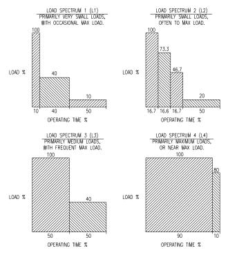
Once the average daily operating time, "t", is calculated for a specific application, the Class of Operating Time can be identified. Using the Class of Operating Time along with the Load Spectrum, one can determine the duty classification requirement of the application. Defining the proposed equipment usage in this manner is critical to selecting the correct hoist for the application.
