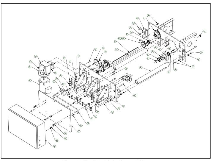
Figure 9-3. Motor Driven Trolley Frame and Drive
