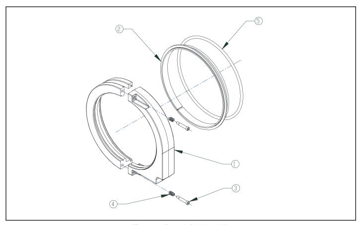
Figure 9-7. Rope Guide Assembly
