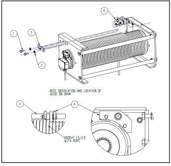
Figure 5-3b. Rope Guide Assembly ("D" Frame)
