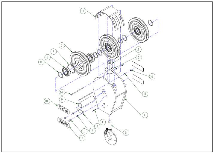
Figure 9-4b. Lower Block Assembly ("D" Frame, 22-1/2t Capacity)
