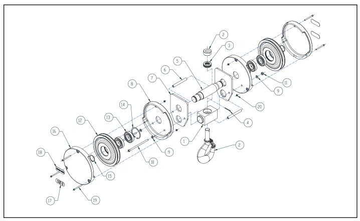
Figure 9-4a. Lower Block Assembly (4-Part Reeving)
