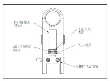
Figure 7-3a. Over-Capacity Limit Switch ("B" & "C" Frames)
