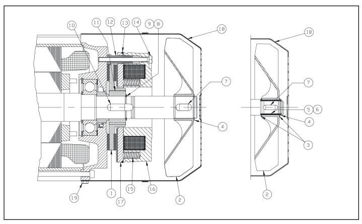
Figure 9-8. Standard Hoist Motor Brake
