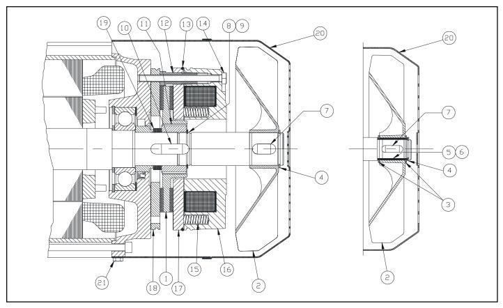
Figure 9-9. Outdoor Service Hoist Motor Brake
