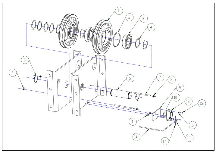
Figure 9-5b. Upper Block Assembly ("D" Frame, 22-1/2t)
