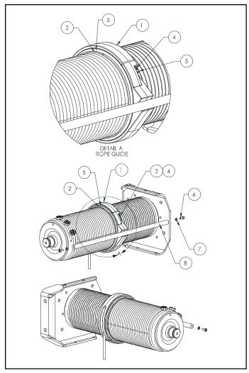
Figure 5-3a. Rope Guide Assembly ("B" & "C" Frame)
