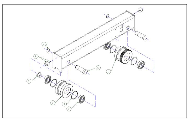
Figure 9-3d. Common Traverse Drive Components ("D" Frame)
