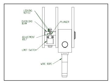
Figure 7-3b. Over-Capacity Limit Switch ("D" Frame)
