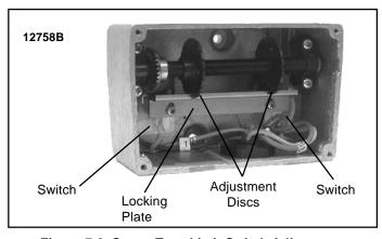
Figure 7-2. Screw-Type Limit Switch Adjustment (Wires Not Shown for Clarity.)
