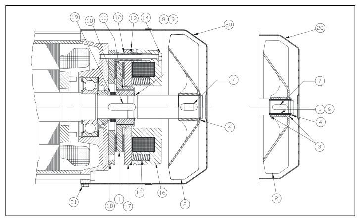
Figure 9-9. Outdoor Service Hoist Motor Brake
