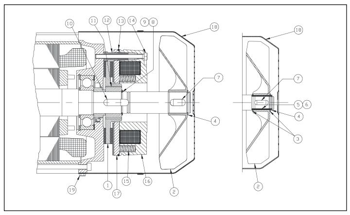
Figure 9-8. Standard Hoist Motor Brake
