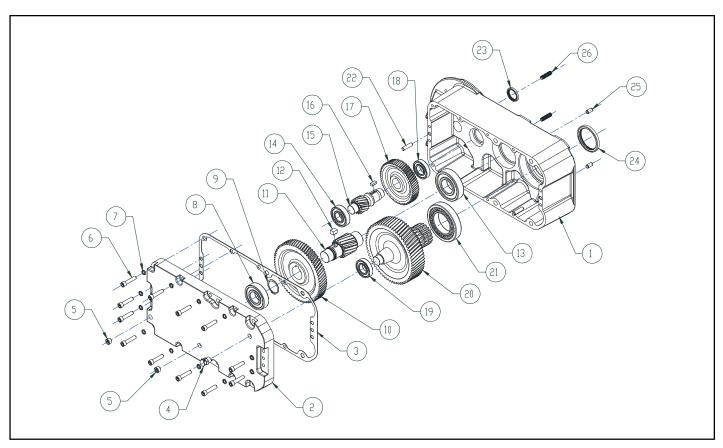
Figure 9-2. Hoist Gearing
