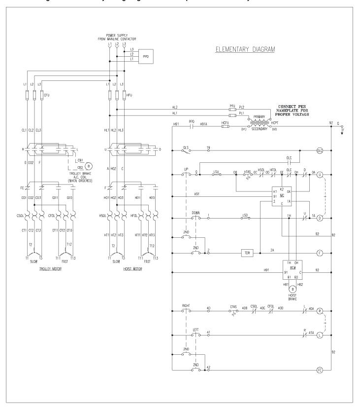
Figure 8-2. Component Diagram for a Two-Speed Hoist and Trolley with Standard Features
