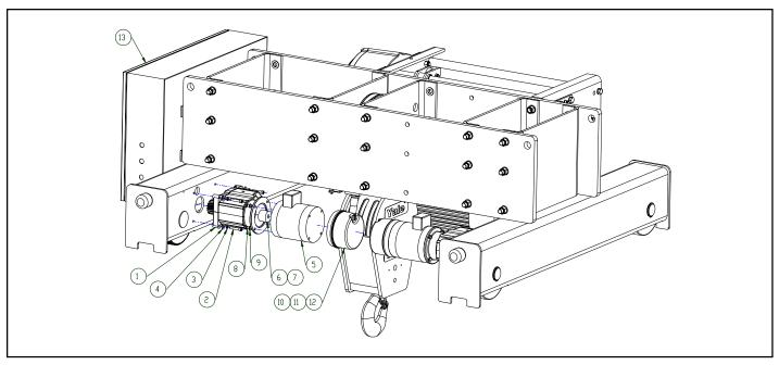
Figure 9-3c. Traverse Drive Component ("D" Frame)
