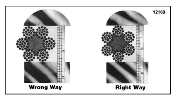
Figure 5-4. Correct Method of Measuring Rope
