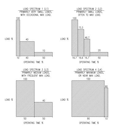
Once the average daily operating time, "t", is calculated for a specific application, the Class of Operating Time can be identified. Using the Class of Operating Time along with the Load Spectrum, one can determine the duty classification requirement of the application. Defining the proposed equipment usage in this manner is critical to selecting the correct hoist for the application.
