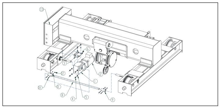
Figure 9-3a. Traverse Drive Component ("B" Frame Shown).
