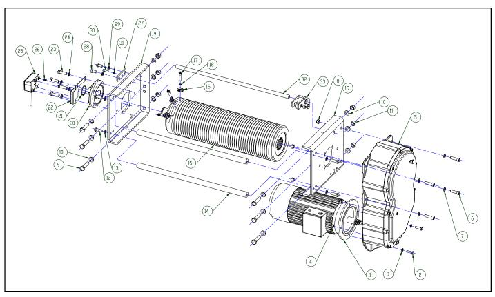
Figure 9-1b. Hoist Drum, Drum Frame, Gearcase, Motor, Rope Guide and Screw Type Limit Switch
