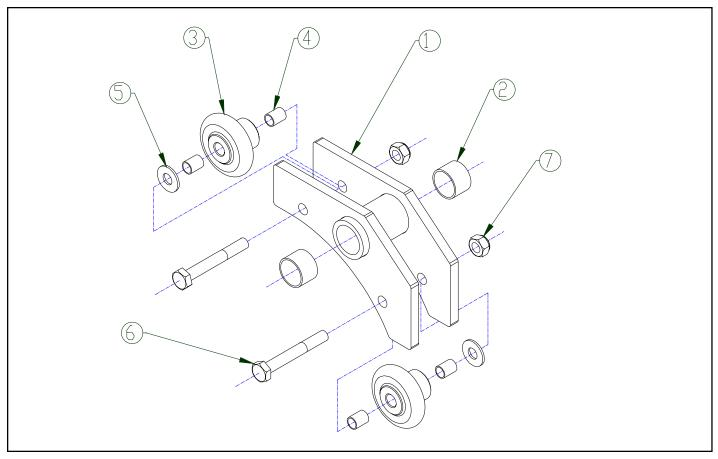
Figure 9-7b. Rope Guide Assembly
