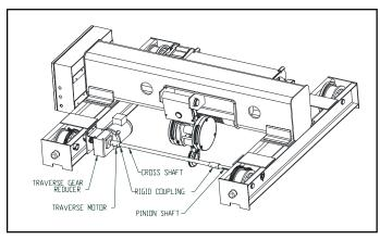
Figure 5-9. Traverse Drive Arrangement ("B" Frame shown above)
