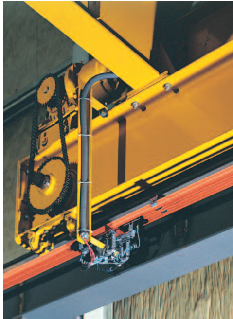
Guide rollers and anti-kickup rollers securely align upper end truck against both sides of track flange.
