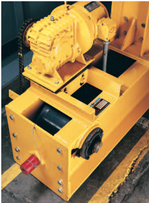
Lower end truck uses large diameter tread wheels. Rotating axle design facilitates easy servicing of wheels, axles, and bearings.
