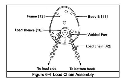
8) Put chain guide [20] (or guide rollers for ½ ton [20-A]) on the frame [13].
