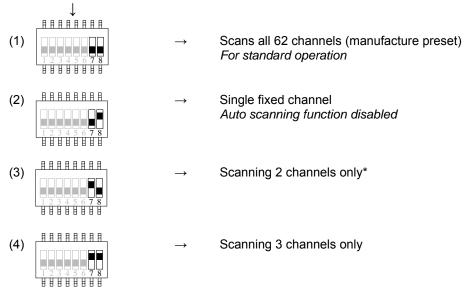
\* If the first 6 dip-switch positions on the receiving module is set to Ch.01 ("000000" or "000001"), when set to 2-channel scanning (type-3 above), then the receiver will only scan Ch.01 and Ch.02.
