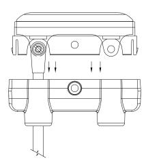
**9.3.(f):** Re-assemble the collector head assembly to the collector with pivot pin and cotter pin. Re-position the shoe into the appropriate conductor.
