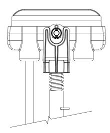
**9.3.(b):** Remove collector head assembly from the collector. To remove the shoe, insert a small flat-headed screwdriver into the slot on the end of the shoe holder and pivot downward.
