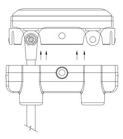
**9.3.(d):** Remove connector hardware from the collector shoe and discard worn collector shoe.
