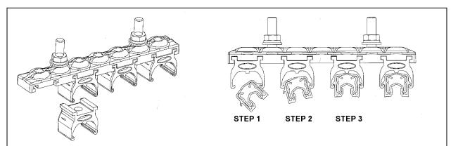
\*INDIVIDUAL HANGERS ARE NOT RE-USABLE. IF REMOVED FROM BASE IT SHOULD BE REPLACED.
