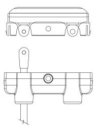
**9.3.(e):** Visually inspect feed cable for any cuts or wear, and replace if necessary. Assemble feed cable to the collector shoe as shown. Push the collector shoe straight into the shoe holder until the shoe sleeve snaps into the shoe holder.
