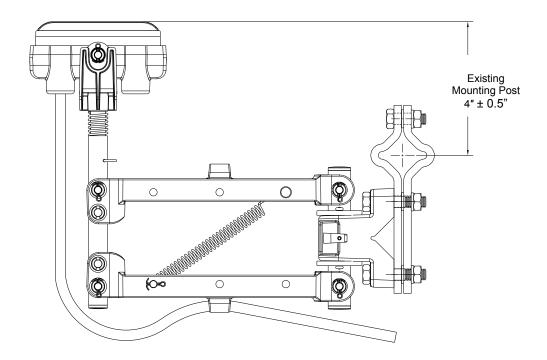
If replacing a single existing collector that is not on the outermost side of the mounting post, it is recommended that the existing collectors are loosened and removed so the new collector can be slid on over the mounting post.
