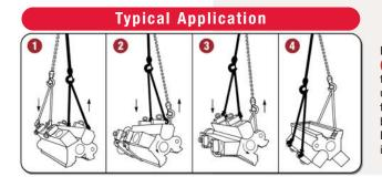
Engine block is raised straight up (1) by special cylinder lift rings, then rotated approximately 45° until one load hook (2) supports total weight. Sling is guided under block and attached to free hook (3). Hoist is then reversed (4) until block is inverted.
