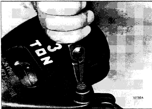
Figure 7-27. Removing Retaining Ring From Bore of Connecting Link Pin — Triple Reeved Lower Block Assembly.
