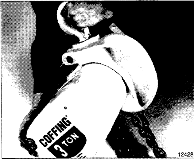
Figure 7-2. Removing 3 Ton Hanger Bracket from Hoist Frame.
