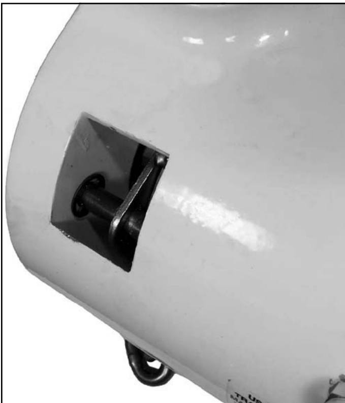
Figure 7-13. Removing Chain Guide Support Pins
