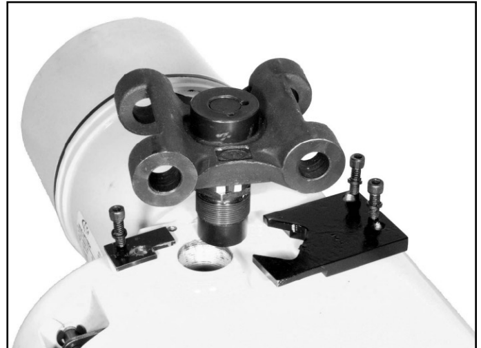
Figure 7-20. Removing Suspension Lug (1/4 through 1 Ton Models)
