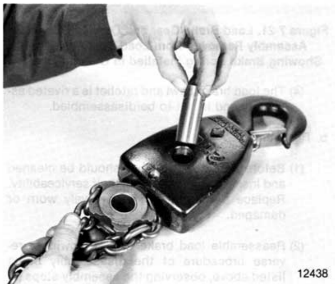
Figure 7-26. Removing Coil Chain and Sprocket on Double and Triple Reeved Lower Block Assembly.
