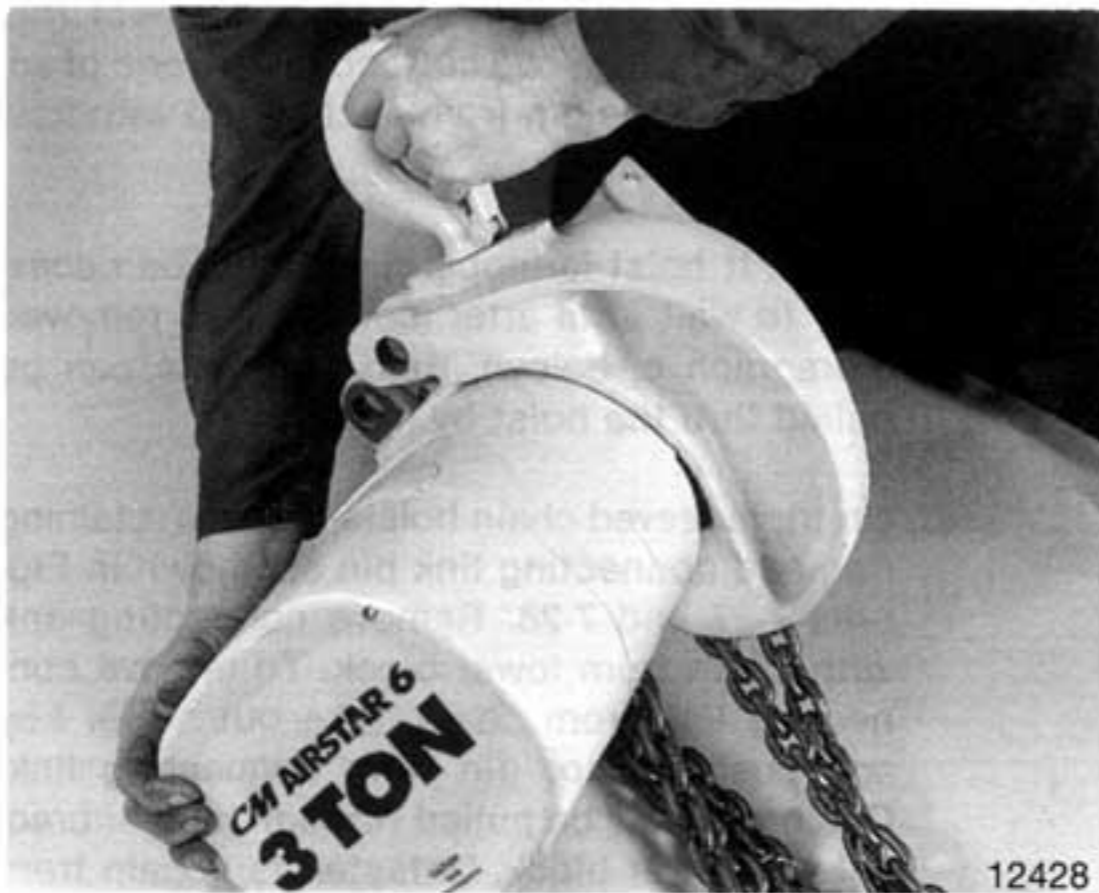
Figure 7-2. Removing 3 Ton Hanger Bracket from Hoist Frame.
