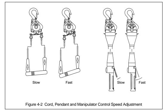
4.4.2 For the pendant or manipulator control, adjust the speed by varying the amount the lever is depressed. As shown in Figure 4-2, by depressing the lever slightly, you will be able to control the hoist's motions slowly and with more precision. By the depressing the lever further, the speed of the hoist will be increased until the lever is fully depressed.
