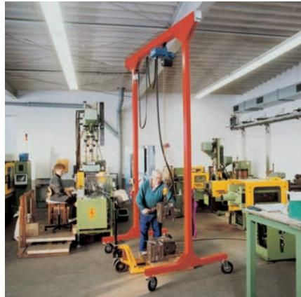
or cannot be installed. They run on solid even surfaces and can be manoeuvred easily in all directions, making them ideal for repair and assembly work.
