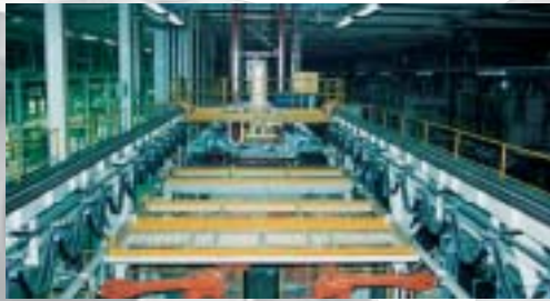
Current supply system on fully automatic automobile welding system
