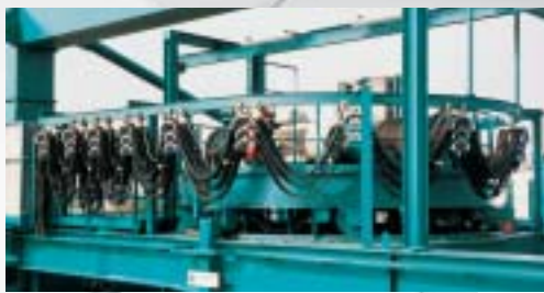
Container crane with rotating crab
