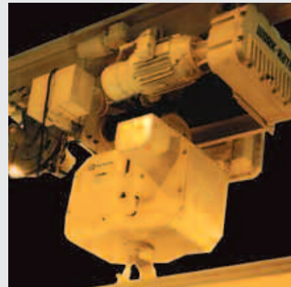
Work-Rated hoist with Mansaver rotating bottom block.
