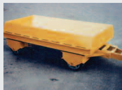
Coil handling trailer.
